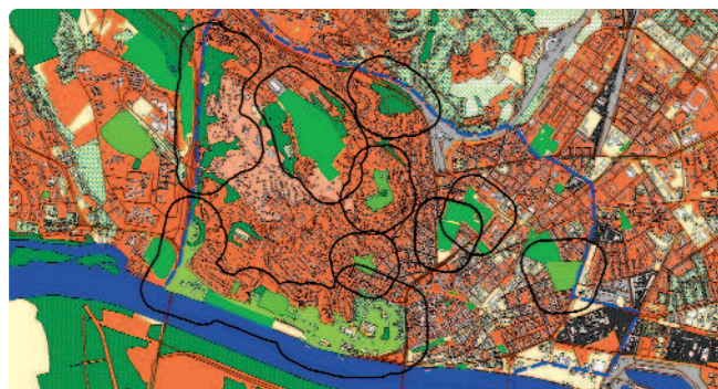
Adaptive capacity of the population to extreme summer heat in Staré Mesto – inhabitants living in the ‘buffer areas’ of green infrastructure have a higher adaptive capacity and therefore lower vulnerability to extreme summer heat
