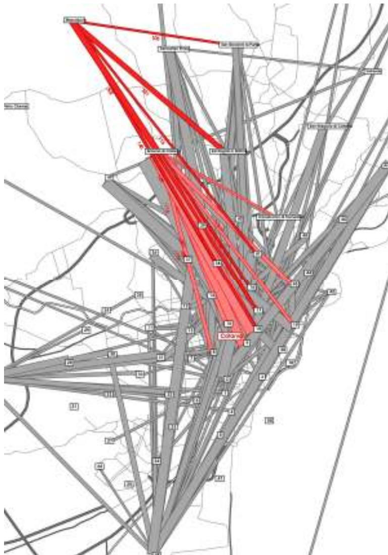
Fig. 8 - Desire lines peak-time commuter traffic (work and study) 6.30-9.00
